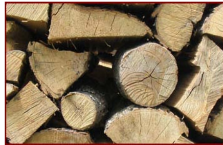
Checks in the end grain of seasoned wood.
